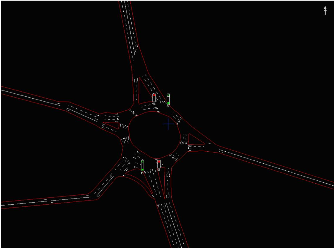
**A585(T) / West Drive junction modelled network** (source: A585(T) Paramics model (Mouchel))
