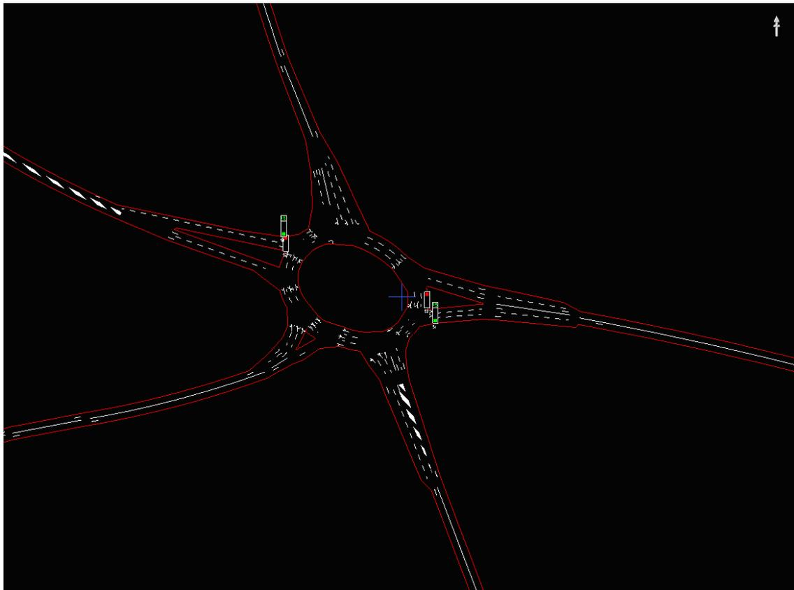
**A585(T) / Anchorsholme Lane junction modelled network** (source: A585(T) Paramics model (Mouchel))
