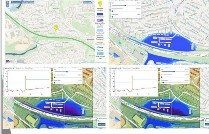
These images show the flooding situation before (in blue) and after (in purple) installing the Andel FloodWall.
