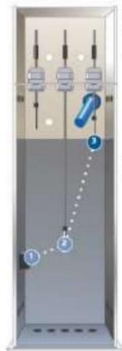
When the rising flood water level reaches the **Start Pump Probe**, the control unit recognises conductivity between **three probes**.
