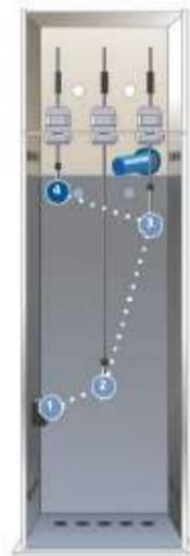
When the rising flood water level reaches the **High Water Alarm Probe**, the control unit recognises conductivity between **four probes**.
