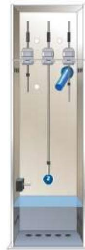
When the receding flood water level falls below the **Stop Pump Probe**, the control unit recognises that there is no conductivity between probes.
